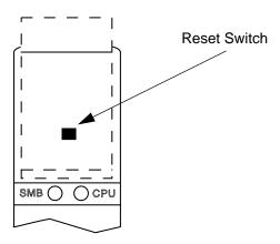
Figure 2-3. The Reset Switch
